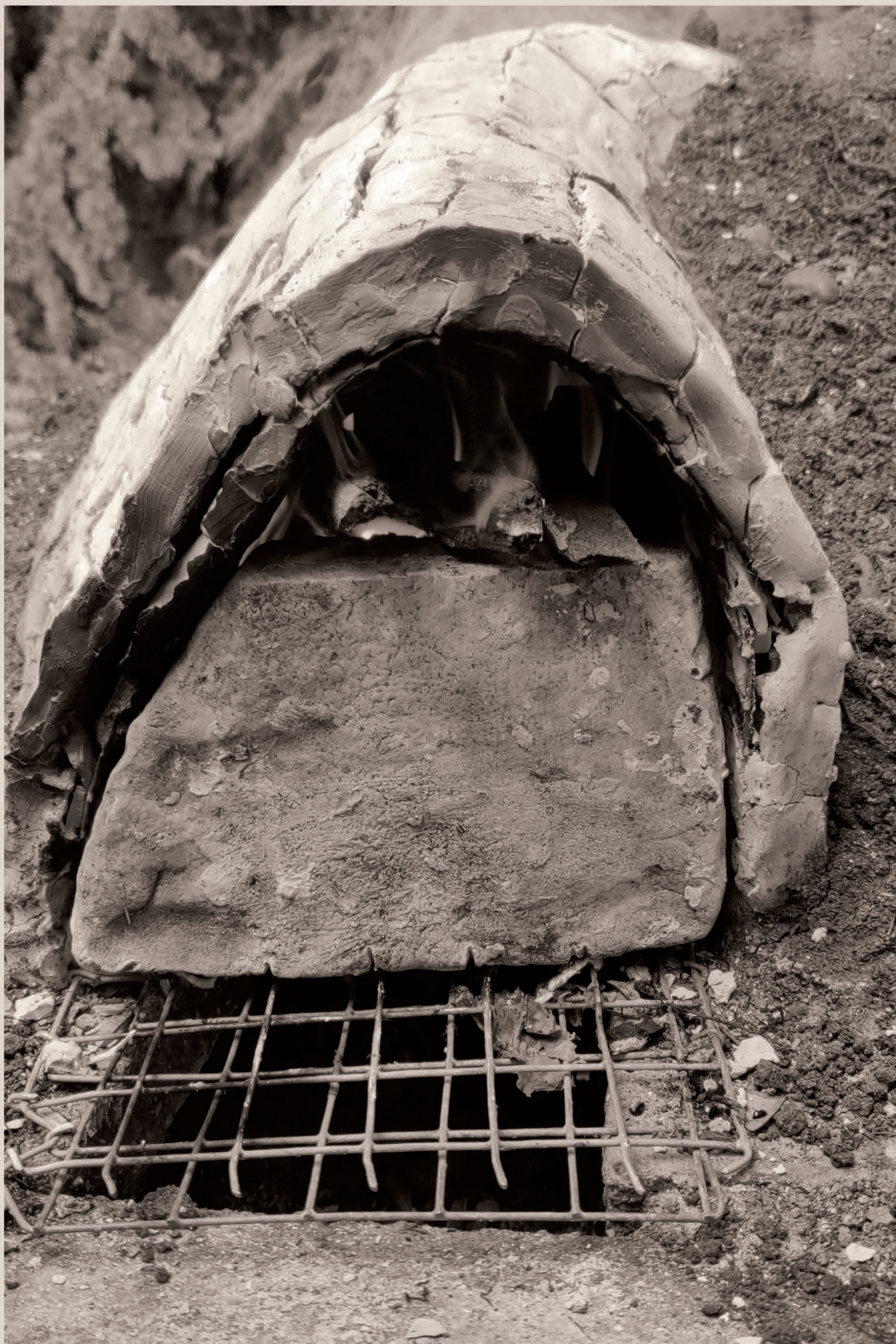
Timber being inserted into the stoke hole, being fed oxygen from the inlet below.
